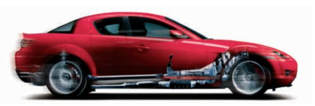
Then, there's the Dynamic Stability Control (DSC), giving the driver the reassurance of intelligent handling by applying appropriate brake-force to individual wheels and managing engine output to prevent skids – without compromising the exciting performance. And for greater cornering control, there's the Limited Slip Differential (LSD), which works with the DSC to help maintain traction while accelerating hard.
